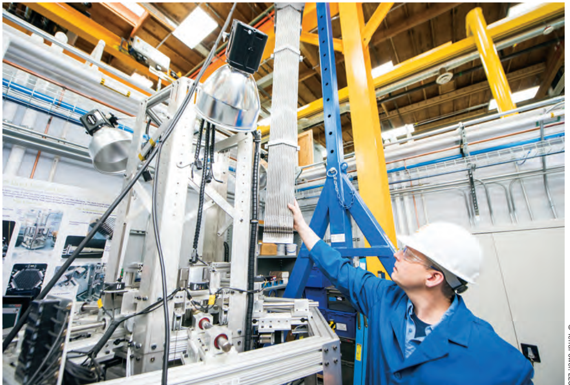
A technician places a full-size test fuel pin bundle in TerraPower's pin duct interaction test apparatus.
